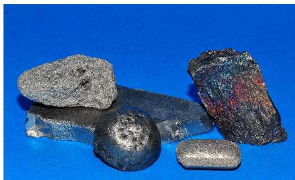
Fig. 2 How elements are added to the molten steel: As pure metals (oxidation level 0 = zero), or as pre-alloys, such as Cr-Fe, Ni-Fe, Mo-Fe etc. In such pre-alloys, the metals are always in oxidation level 0.
