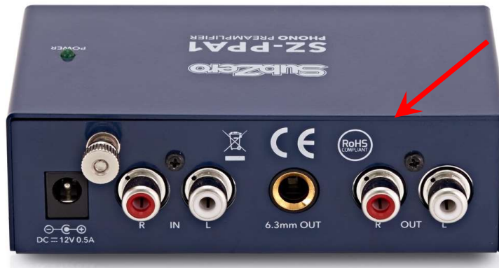
Fig. 1 Where the RoHS label is relevant: Electronic parts, here a small pre-amplifier connecting a traditional turntable with the amplifier. The red arrow shows the RoHS logo.
