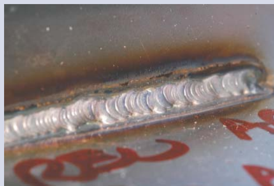
Welded sample of "acid resistant" ferritic 4521. Thickness: 2 mm; method: TIG; filler metal: AISI 316LSi; current: 90 A; and purge gas: pure Ar.
